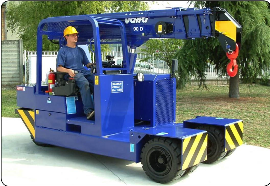
**ENGINE:** Diesel 51 HP, 4 cylinders, water cooled with electric starter and automatic fuel switch off.
